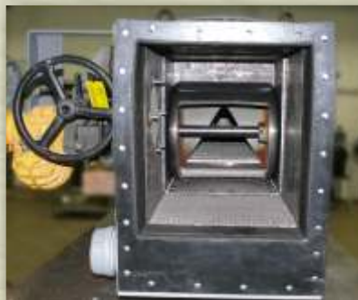
The rotary control valve varies the reclaim rate by comparing a weigh-scale signal with the desired discharge rate.
