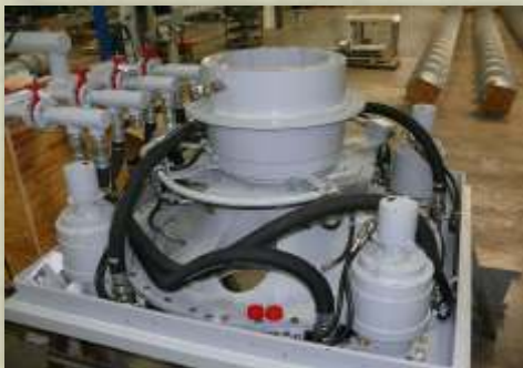
The fully-aerated center section and discharge chute prevents hard-pack formation if material is stored for an extended time without reclamation.
