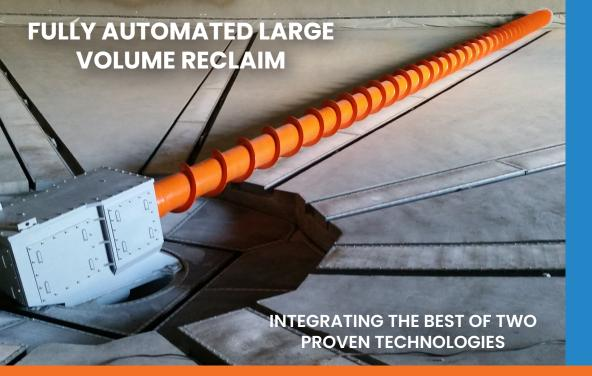
Laidig's Fluidized Screw reclaim systems are designed specifically for heavy-duty applications requiring high-volume storage and reclaim of fluidizable materials.
