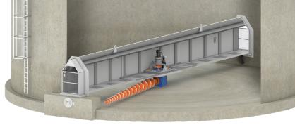
The Planetaire provides an access beam which spans the entire diameter of the storage vessel. This beam offers complete access to all components of the Planetaire, even under a full head-height of material. Serviceable components would include motors, gearboxes, reducers, and the auger cutter blades. Even the entire auger can be removed from a full silo through one of the auger access doors at the end of the beam.
